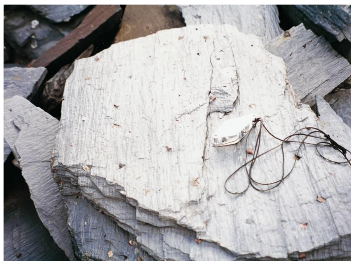
Figure 6 Easdale is a blue grey slate often with a crinkly surface. In this example the crystals of pyrite are unchanged after years of weathering,
