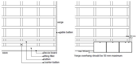
Fig A - Batten configuration
