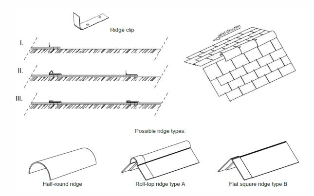
In case dry ridges are used in another material (concrete, clay, sheet metal ridges), they should be laid in accordance with the slate and/or the sheet metal manufacturer's technical recommendations.
