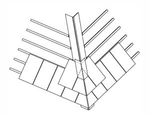
Cut slates to a close mitre to the hip line. Use wide slates (cut from doubles) rather than using small pieces of slate, for all but the steepest pitches. This ensures that the raking cut provides enough width at the head of the slates to resist wind uplift.
