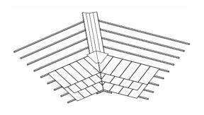
Cut the slates to a close mitre to the valley line. Make sure the tail of the slates is always wide enough. Use wide slates (cut from doubles) rather than using small pieces of slate.
