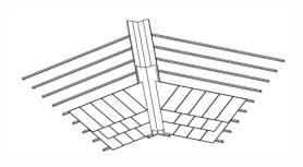
On both sides of the valley line a timber lay-board is applied. On top of these a sheet metal valley is laid, fully supported on lay-boards with a thickness of minimum 19 mm.
