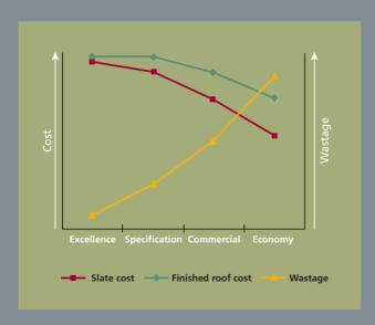
Note: all natural slates must be sorted prior to installation in accordance with BS 8000-6: 2013. When deciding on the most appropriate slate we recommend that you consider all of the costs associated. These include wastage rates, grading, sorting and trimming required with the lesser quality slates along
